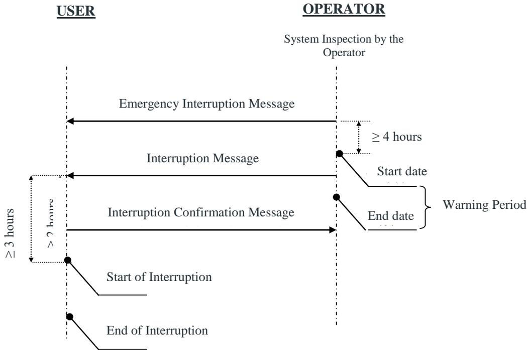
2. The Emergency Interruption Procedure at an NNGTS Entry Point/Reverse Flow Entry Point is summarised in the figure below:
